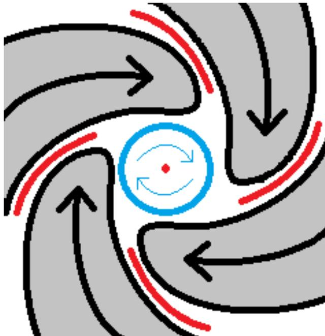
In trapping, which may be the most important criteria where the polywell fails, the NESAR has at least two levels of improvement. First, the NESAR improves upon the polywell by pushing the confined electrons in a way that completely bypasses the magnetic field cusps where electrons can escape.
